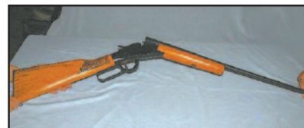
Ithica M-66 Super Single .410 ga; Lever Action; Exposed Hammer; 3" chamber; full choke
