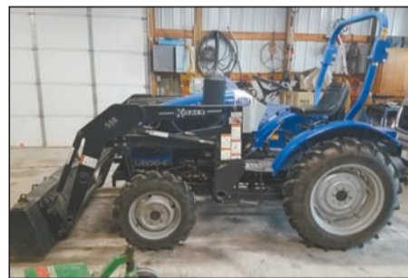
Lenar LE 274-1 MFWD compact tractor with Koyker 140 quick attach loader, 3 pt, 540 rpm PTO
